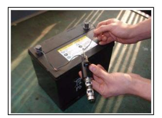
3. When 12V power is provided to the OCV, the OCV must move forward as shown in the picture to the right.
